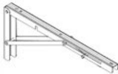
2094 FOLDING TABLE BRACKET - A4M02094 (x2) 1 3/8"x6 13/16"x15 15/16" (34x173x405)
