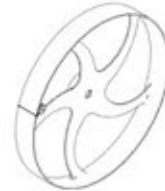
W01 WHEEL ASSEMBLY - A4M02146 (x1) 2 3/8"x7" (59.7x178)
