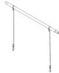
S01 SPINDLE ASSEMBLY - A4M02150 (x1) (1 3/16"x37 1/2") (30x955)
