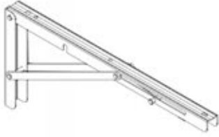
2094 SUPPORT DE TABLE PLIANTE - A4M02094 (x2) 1 3/8"x6 13/16"x15 15/16" (34x173x405)
