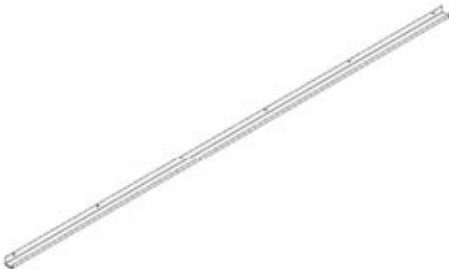
G02 GUTTER - A4M02583 (x4) 1 9/16"x1 15/16"x111" (40x50x2819)
