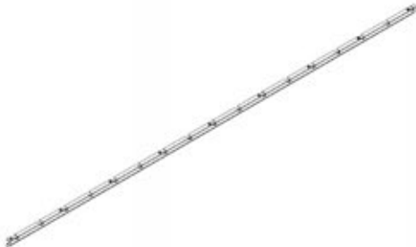
M01 LOUVER MOUNT - A4M02593 (x1) 1"x1 15/16"x110 3/4" (25x49x2813)
