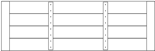
RP01 ROOF PANEL - W2A04246 (x4) 1 3/8"x19 3/8"x46 3/4" (35x370x1137)
