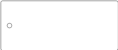
NG01 LOWER RIGHT WALL RAIL - W4L21488 (x1) 3/4"x3 3/8"x8" (20x86x203)
