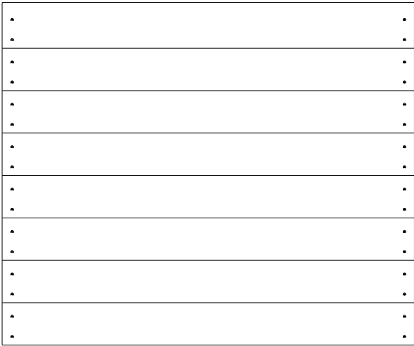
RP01 ROOF PANEL - W2A04295 (x2) 1 5/8"x40 7/8"x49 3/16" (42x1038x1250)
