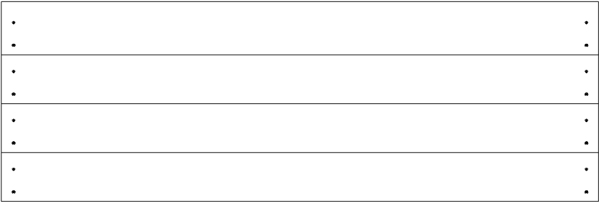
RP2 ROOF PANEL - W2A04273 (x2) 1 5/8"x20 5/8"x66" (42x540x1613)
