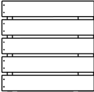
BA04 OUTSIDE BENCH ASSEMBLY - W2A04808 (x1) 1 15/16"x19 3/16"x19 3/4" (50x487x502)
