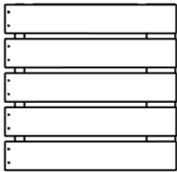
BA03 OUTSIDE BENCH ASSEMBLY - W2A04806 (x1) 1 15/16"x19 1/8"x19 3/4" (50x486x502)
