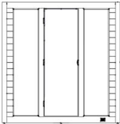
P07 FRONT PANEL - W2A04840 (x1) 76 15/16"x74 13/16"x2 3/8" (60x1901x1954)
