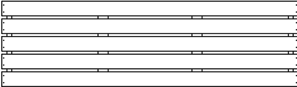
BA02 BENCH ASSEMBLY-W2A04928 (x1) 1 15/16"x19 1/8"x65 3/4" (50x486x1670)
