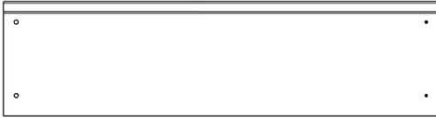
OJ03 WALL BOARD - W4L22471 (x1) 1 3/16"x5 1/4"x20 1/8" (30x134x511)
