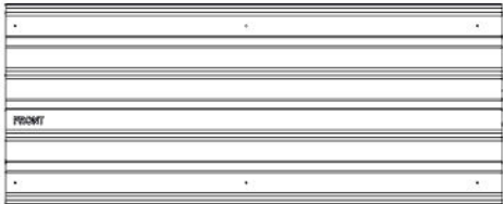
3113 29GA STEEL SHEETING - A4M03113 (x8) 1/4"x18 7/8"x46 7/16" (7x480x1179)
