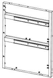
S5 SIDE PANEL ASSEMBLY - A4M05460 (x1) 33 3/4"x25"x1 3/8" (35x635.0x857)
