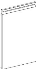
D6 DOOR ASSEMBLY - A4M05471 (x1) 22 3/8"x15 1/2"x7/8" (22x393.5x569)
