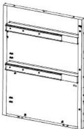
S4 SIDE PANEL ASSEMBLY - A4M05458 (x1) 33 3/4"x25"x2 11/16" (68x635x857)
