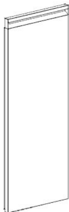
D8 DOOR ASSEMBLY - A4M05480 (x1) 33 1/2"x12 11/16"x7/8" (22x324.1x851)
