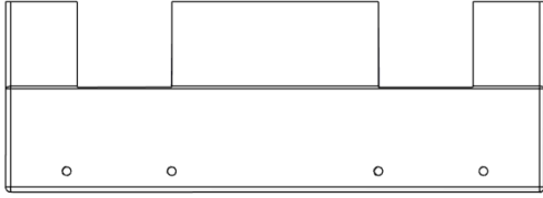
AL01 BASE RAMP W/ PRODUCT ID TAG - W2A05123 (x1) 1 7/16"x4 5/16"x12 1/8" (36x109x308)
