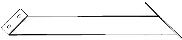
F2 | LONG ANGLE BRACE - A4M01274 (2) | 1 1/8"x4"x21 1/2" (30x101x546)
