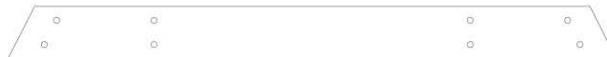
M82 PLANCHE DE SOL DE BARRE DE SINGE - W4L13850 (1) 5/8"x3 3/8"x39 5/8" (16x86x1006)
