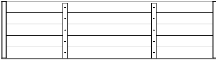
(1) RP3 - ROOF PANEL - W2A01862 1 3/8"x16 1/8"x59 1/2" (35x410x1532)
