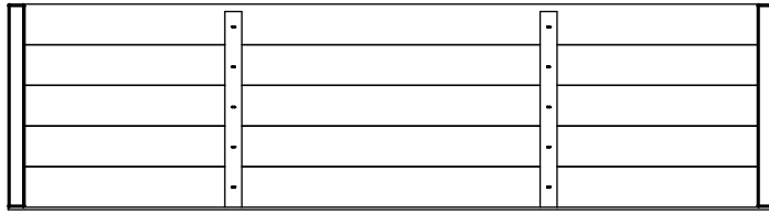
(1) RP3 - ROOF PANEL - W2A01862 1 3/8"x16 1/8"x59 1/2" (35x410x1532)
