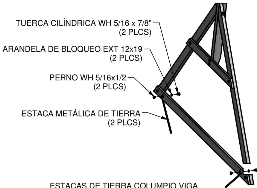
ESTACAS DE TIERRA COLUMPIO VIGA
