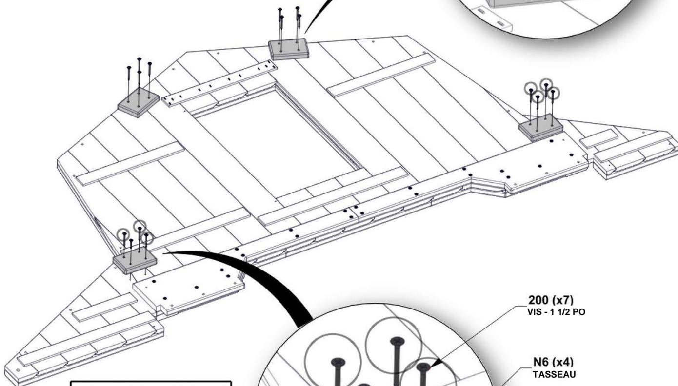
REMARQUE : LA VIS COURTE DE 1 PO DOIT ALLER DANS L'EMPLACEMENT SPÉCIFIÉ.
