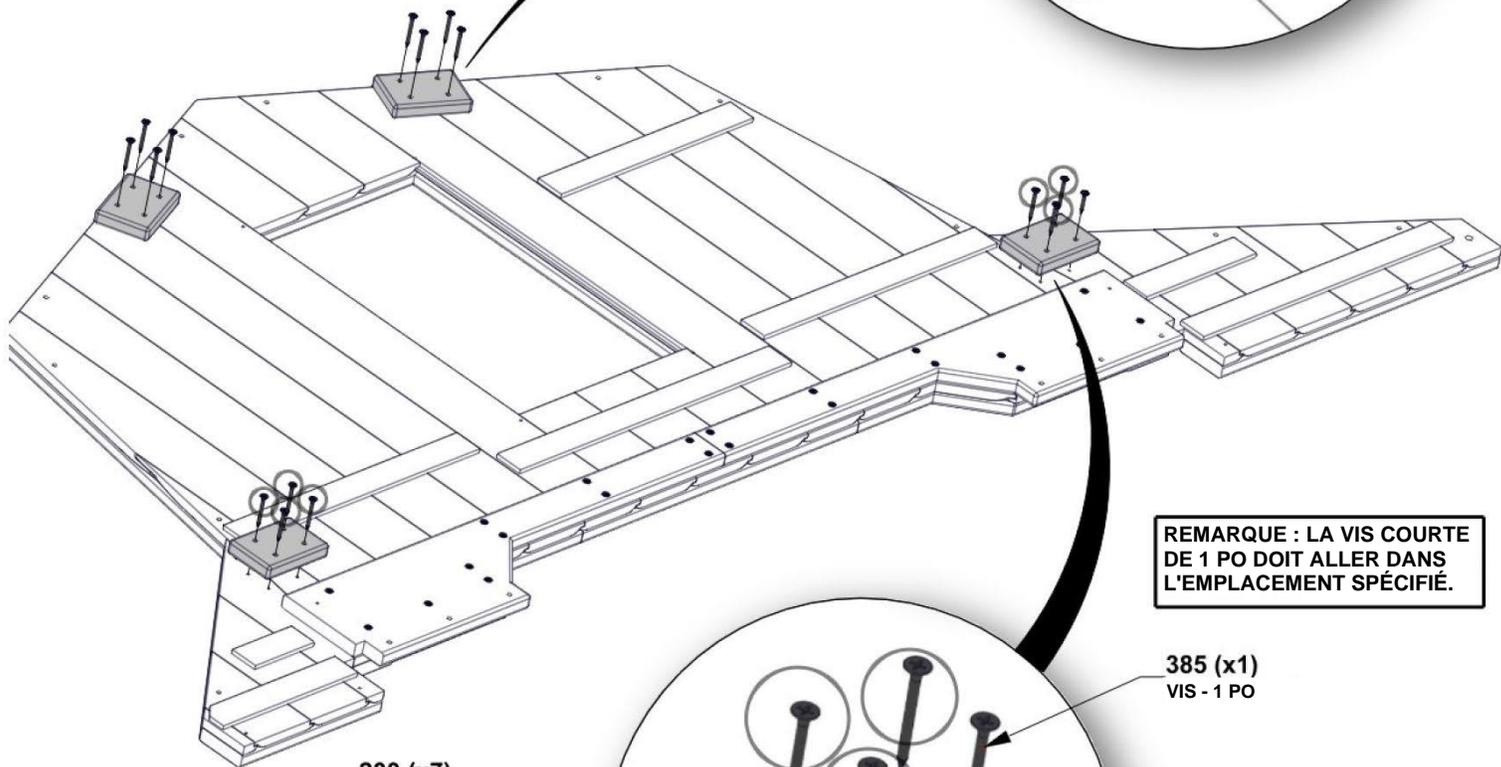
**REMARQUE : LA VIS COURTE DE 1 PO DOIT ALLER DANS L'EMPLACEMENT SPÉCIFIÉ.**
