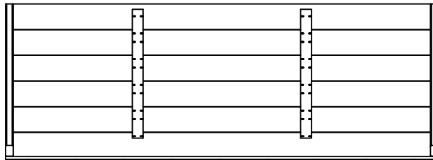
(2) RP1 - ROOF PANEL - W2A01677 1 3/4"x19 1/4"x53 3/4" (45x490x1366)
