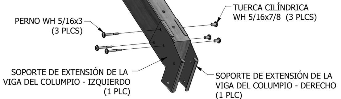
(1) **SP50 - SOPORTE DE LA VIGA DEL COLUMPIO - W102417 - 3 3/8"x3 3/8"x49 3/8" (86x86x1254)**
