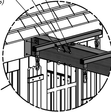
ENSAMBLAJE DE VIGA DEL COLUMPIO
