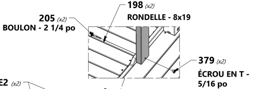
NOTER L'ORIENTATION DU TROU POUR UN MONTAGE CORRECT.
