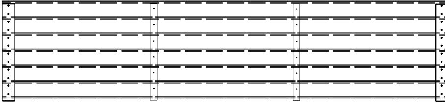
RP02 | PANEL DE TECHO - W2A020184 (x1) | 1 9/16"x19 1/4"x85 3/16" (40x488x2165)
