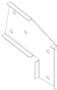
(1) SOPORTE DERECHO EXT. DE LA VIGA DEL COLUMPIO COLOR AZUL - A4M00512
