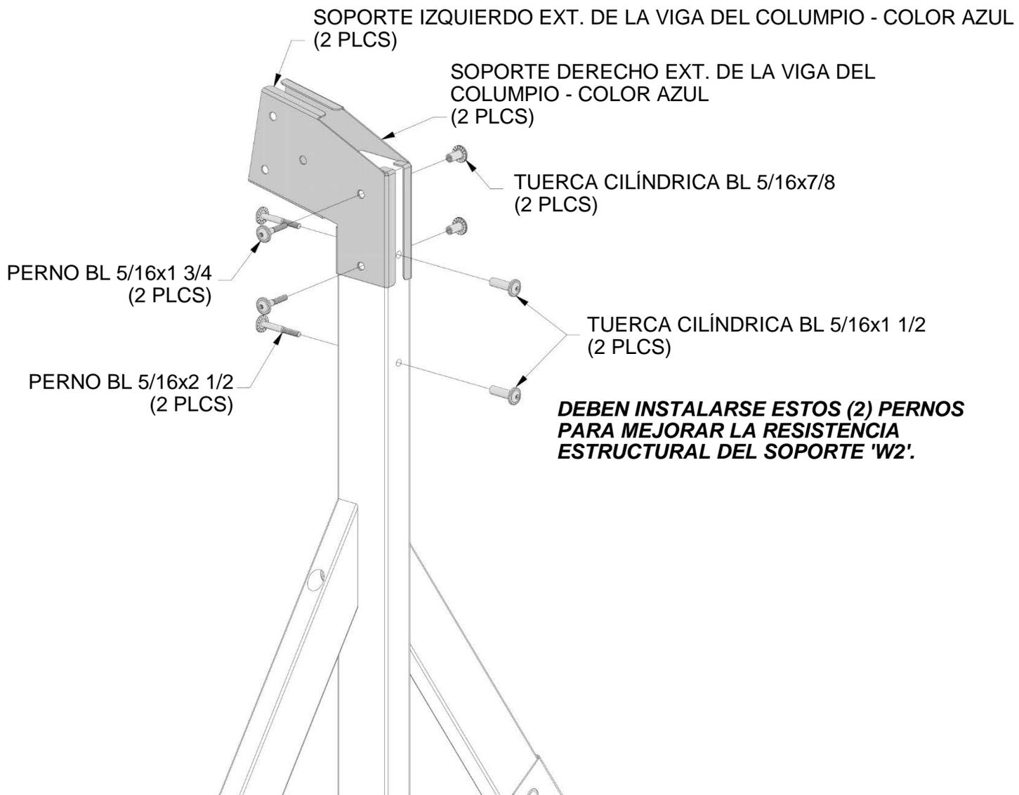
**MONTAJE DE LA VIGA DEL COLUMPIO**
