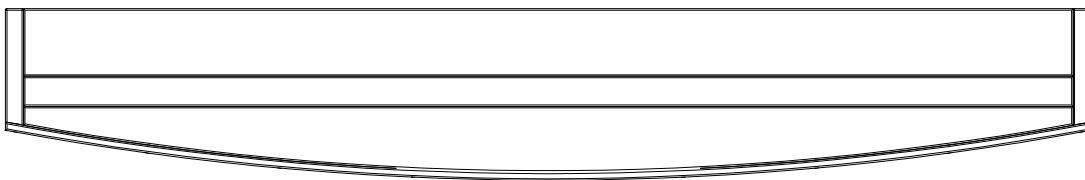
(1) TT1 - INSIDE TABLE TOP ASSEMBLY - W2A02564 2 3/8"x13 3/8"x84 7/8" (60x340x2156)
