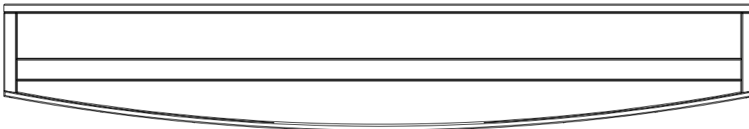
(1) TT2 - OUTER TABLE TOP ASSEMBLY - W2A02811 2 3/8"x14 5/16"x84 7/8" (60x364x2156)
