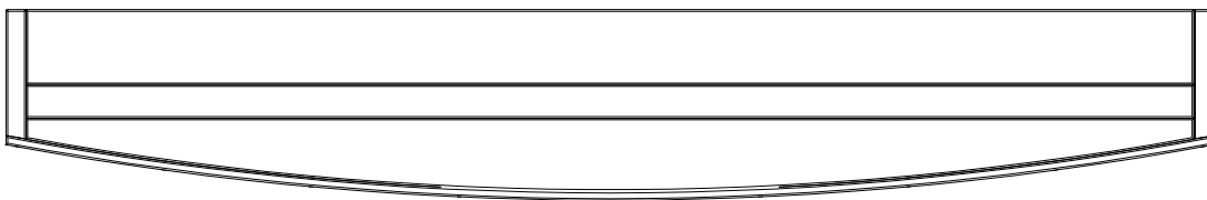
(1) TT1 - INSIDE TABLE TOP ASSEMBLY - W2A02812 2 3/8"x13 3/8"x84 7/8" (60x340x2156)
