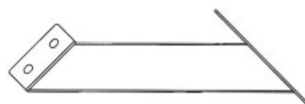
F4 | SHORT ANGLE BRACE - A4M01276 (2) 1\frac{1}{8} \times 4 \times 14 (30x101x355)
