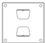
G1 | POST FOOT PLATE - A4M01278 (4) | 2 1/8"x8 3/8"x8 3/8" (54x213x213)
