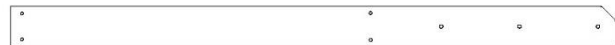
G1 | PLANCHE AU SOL - W4L13582 (x1) | 1 po x 5 1/4 po x 79 1/8 po (24x134x2010)
