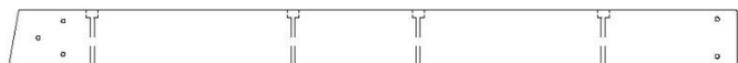
SB74 POUTRE DE BALANÇOIRE 2 POSITIONS - W4L13780 (x1) 2 po x 5 1/4 po x 68 3/4 po (50x134x1745)
