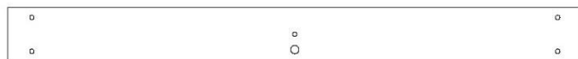
K5 | PLANCHE AU SOL - W4L13757 (x1) | 5/8 po x 4 3/4 po x 50 1/4 po (16x120x1275)
