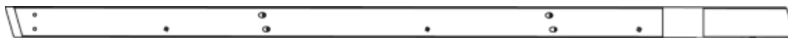
H01 | SOLIVE DE TOIT - W4L16295 (2) | 1 po x 3 3/8 po x 88 3/16 po (24 x 86 x 2240)
