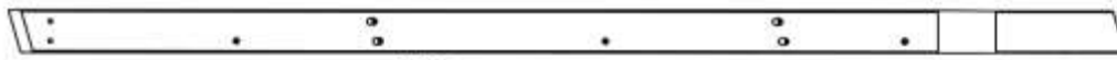
H01 | SOLIVE DE TOIT - W4L16295 (1) | 1 po x 3 3/8 po x 88 3/16 po (24 x 86 x 2 240)
