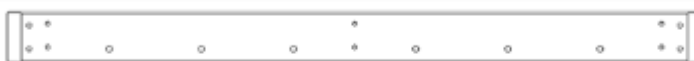
H02 | SOLIVE DE TOIT - W4L16283 (2) | 1 po x 3 3/8 po x 46 3/4 po (24 x 86 x 1188)
