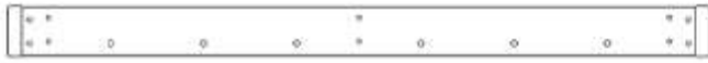
H02 | SOLIVE DE TOIT - W4L16283 (1) | 1 po x 3 3/8 po x 46 3/4 po (24 x 86 x 1 188)
