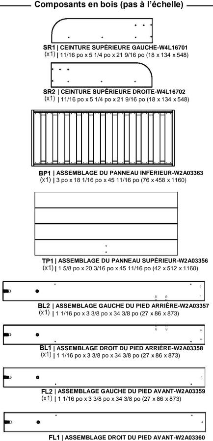
**FL1 | ASSEMBLAGE DROIT DU PIED AVANT-W2A03360** (x1) | 1 1/16 po x 3 3/8 po x 34 3/8 po (27 x 86 x 873)
