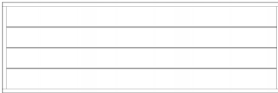
TP1 TOP PANEL ASSEMBLY - W2A03348 (x1) 2 15/16"x16 5/8"x50 11/16" (75x423x1288)
