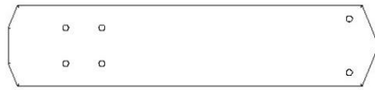
D01 | PLANCHE DE RIVE DU PIGNON - W4L16850 (x1) | 1 3/8 po x 5 1/4 po x 24 1/4 po (36x134x615)
