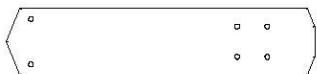
D01 | PLANCHE DE RIVE DU PIGNON - W4L16850 (x4) | 1 3/8 po x 5 1/4 po x 24 1/4 po (36x134x615)
