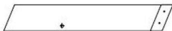
E07 | CHEVRON - W4L15209 (2) | 1\frac{3}{8} po x 3\frac{3}{8} po x 21\frac{15}{16} po (36x86x557)
