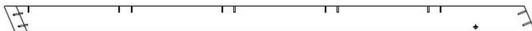
E02 | CHEVRON - W4L15290 (2) | 1\frac{3}{8} po x 3\frac{3}{8} po x 67\frac{1}{8} po (36x86x1705)
