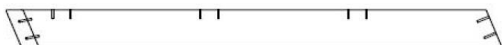
E03 | CHEVRON - W4L15291 (2) | 1\frac{3}{8} po x 3\frac{3}{8} po x 43\frac{5}{8} po (36x86x1109)
