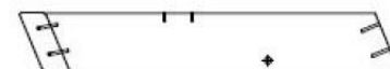
E13 | CHEVRON - W4L15219 (2) | 1\frac{3}{8} po x 3\frac{3}{8} po x 21\frac{15}{16} po (36x86x557)
