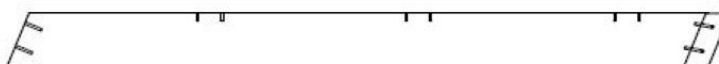
E06 | CHEVRON - W4L15208 (2) | 1\frac{3}{8} po x 3\frac{3}{8} po x 45\frac{7}{16} po (36x86x1155)
