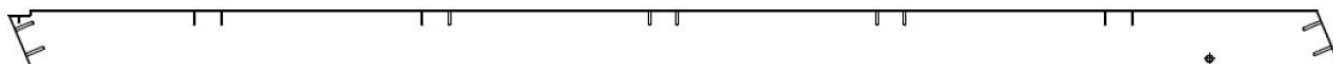
E14 | CHEVRON - W4L15299 (2) | 1\frac{3}{8} po x 3\frac{3}{8} po x 76\frac{11}{16} po (36x86x1948)
