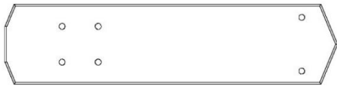
D03 PLANCHE DE RIVE DU PIGNON - W4L17202 (x1) 1 3/8 po x 5 1/4 po x 21 3/4 po (36x134x553)
