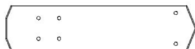
D03 PLANCHE DE RIVE DU PIGNON - W4L17202 (x4) 1 3/8 po x 5 1/4 po x 21 3/4 po (36x134x553)
