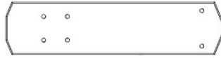
D03 PLANCHE DE RIVE DU PIGNON - (x1) W4L17202 1 3/8 po x 5 1/4 po x 21 3/4 po (36x134x553)
