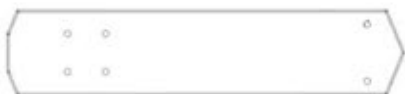
D01 PLANCHE DE RIVE DU PIGNON - W4L16415 (x8) 1 3/8 po x 5 1/4 po x 24 5/8 po (36x134x625)
