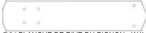
D01 PLANCHE DE RIVE DU PIGNON - W4L16415 (x1) 1 3/8 po x 5 1/4 po x 24 5/8 po (36x134x625)
