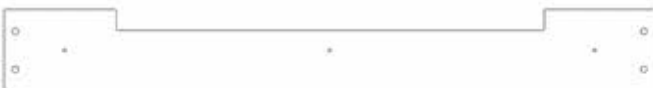
G10 Riel de Pared del Balcón Delantero - W4L17649 (x1) 1"x5 1/4"x40 5/8" (24x134x1032)
