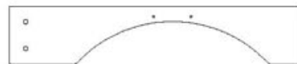
D02 LISSE TUNNEL - W4L17726 (x1) 1 3/8 po x 5 1/4 po x 26 3/4 po (36 x 134 x 681)
