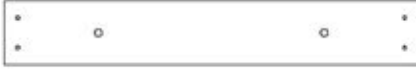
H102 PLANCHE DE FIXATION - W4L17928 (x1) 1 po x 3 3/8 po x 21 5/8 po (24 x 86 x 550)
