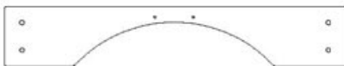
D01 LISSE TUNNEL - W4L17725 (x1) 1 3/8 po x 5 1/4 po x 30 1/4 po (36 x 134 x 767)
