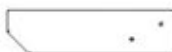
H19 SUPPORT DE TABLE - W4L17981 (x1) 1 po x 2 3/4 po x 10 1/2 po (24 x 70 x 268)
