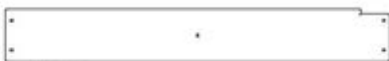
L02 PLANCHE DE PLANCHER - W4L17761 (x1) 5/8 po x 4 3/8 po x 32 1/8 po (16 x 112 x 815)
