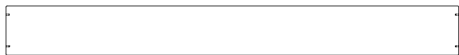
G19 PLANCHE DE SUPPORT - W4L17966 (x1) 1 po x 5 1/4 po x 48 1/4 po (24 x 134 x 1226)
