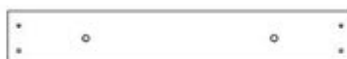
H102 PLANCHE DE FIXATION - W4L17928 (x1) 1 po x 3 3/8 po x 21 5/8 po (24 x 86 x 550)
