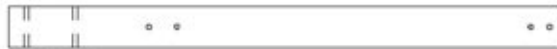
SP71 SUPPORT DE POUTRE DE BALANÇOIRE - W4L17937 (x1) 3 3/8 po x 3 3/8 po x 46 1/8 po (86 x 86 x 1172)
