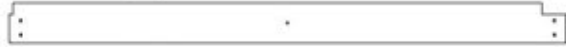
M05 PLANCHE MURALE - W4L17748 (x1) 5/8 po x 3 3/8 po x 46 1/2 po (16 x 86 x 1182)
