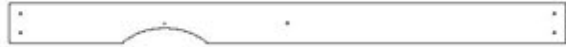
M06 PLANCHE MURALE - W4L17749 (x2) 5/8 po x 3 3/8 po x 46 1/2 po (16 x 86 x 1182)
