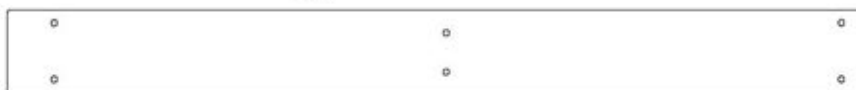
G16 LISSE MURALE - W4L17738 (x1) 1 po x 5 1/4 po x 54 po (24 x 134 x 1372)
