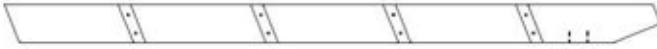
E74 MONTANT GAUCHE - W4L17924 (x1) 1 3/8 po x 3 3/8 po x 57 1/4 po (36 x 86 x 1453)
