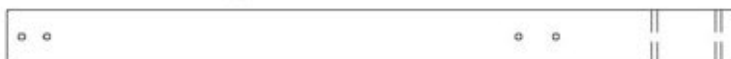
SP71 SUPPORT DE POUTRE DE BALANÇOIRE - W4L17937 (x1) 3 3/8 po x 3 3/8 po x 46 1/8 po (86 x 86 x 1172)
