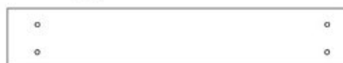
G18 SUPPORT DE PLANCHER - W4L17754 (x1) 1 po x 5 1/4 po x 29 7/8 po (24 x 134 x 758)
