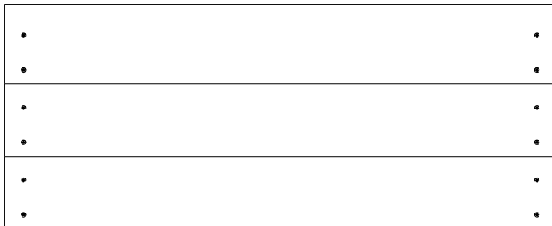
RP5 ROOF PANEL - W2A03760 (x2) 1 5/8"x15 5/8"x59" (42x396x974)
