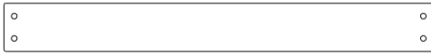
H21 RAIL MURAL DU NID DE CORBEAU - W4L18300 (x1) 1"x3 3/8"x29 7/8" (24x86x758)
