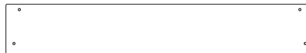
L04 RAIL MURAL DU NID DE CORBEAU - W4L18296 (x1) 5/8"x4 3/8"x27" (16x112x686)
