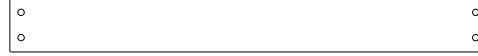
M06 RAIL MURAL DU NID DE CORBEAU - W4L18302 (x2) 5/8"x3 3/8"x29 7/8" (16x86x758)
