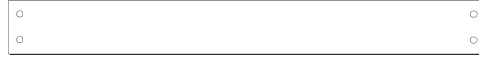
H21 RAIL MURAL DU NID DE CORBEAU - W4L18300 (x2) 1"x3 3/8"x29 7/8" (24x86x758)
