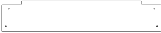
L05 RAIL MURAL DU NID DE CORBEAU - W4L18306 (x1) 5/8"x5 1/4"x27" (16x134x686)
