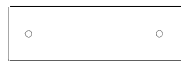
H24 RAIL MURAL DU NID DE CORBEAU - W4L18304 (x2) 1"x3 3/8"x11 1/8" (24x86x282)
