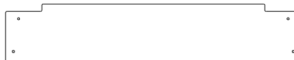
L05 RAIL MURAL DU NID DE CORBEAU - W4L18306 (x1) 5/8"x5 1/4"x27" (16x134x686)
