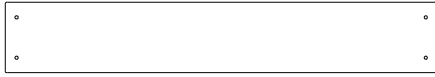
L03 RAIL MURAL DU NID DE CORBEAU - W4L18295 (x6) 5/8"x4 3/8"x27" (16x112x686)
