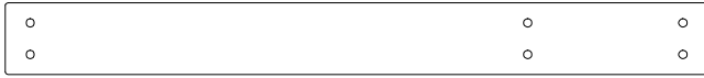
E03 RAIL DE SOL DU NID DE CORBEAU - W4L18291 (x2) 1 3/8"x3 3/8"x33 1/4" (36x86x846)
