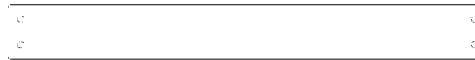
M06 RAIL MURAL DU NID DE CORBEAU - W4L18302 (x2) 5/8"x3 3/8"x29 7/8" (16x86x758)
