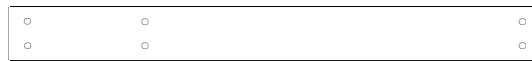
E03 RAIL DE SOL DU NID DE CORBEAU - W4L18291 (x2) 1 3/8"x3 3/8"x33 1/4" (36x86x846)
