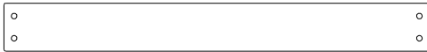
H21 RAIL MURAL DU NID DE CORBEAU - W4L18300 (x1) 1"x3 3/8"x29 7/8" (24x86x758)
