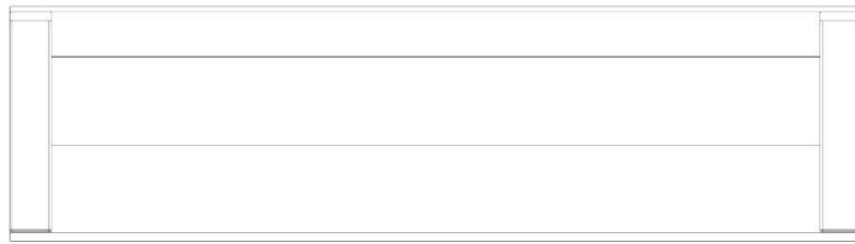
RP1 PANEL SUPERIOR DEL TECHO - W2A03948 (x2) 1 5/8"x13 3/8"x48 7/8" (42x341x1241)
