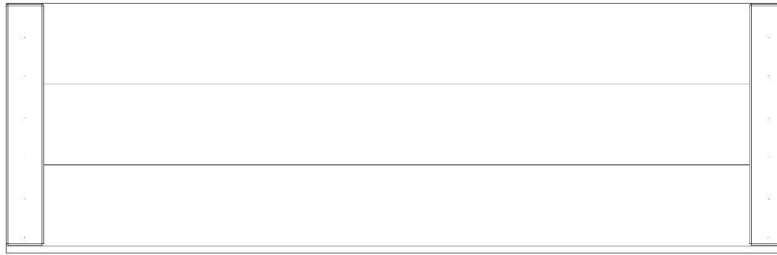
RP2 PANEL DE TECHO - W2A03947 (x2) 1 5/8"x15 5/8"x59 3/8" (42x396x1241)
