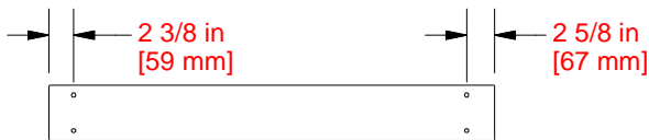
G02 GROUND BOARD - W4L19064 (x1) 1"x5 1/4"x42 1/4" (24x134x1072)
