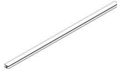
A2 VERTICAL SUPPORT - A4M02039 (x1) 1 15/16"X1 3/16"X57 7/8" (30x50x1470)
