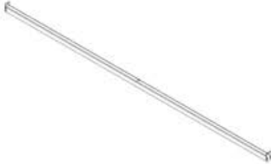
A1 HORIZONTAL BRACE ASSEMBLY - A4M01806 (x2) 1 7/16"X2 5/16"X88" (36x58x2235)
