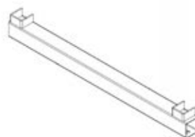
F09 BOTTOM FLOOR TUBE - A4M02210 (x1) 1 9/16"x2 3/8"x21 7/8" (40x60x555)
