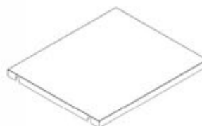
F10 FLOOR PANEL - A4M02208 (x1) 1 3/16"x18 3/8"x21 3/4" (30x467x553)
