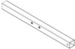
F06 TABLE TUBE SUPPORT - A4M02205 (x1) 1 9/16"x1 9/16"x21 7/8" (40x40x555)
