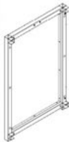
C01 CABINET PANEL - A4M02016 (x1) 2 3/4"x25"x38" (70x635x965)
