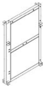
C02 CABINET PANEL - A4M02017 (x1) 3 15/16"x25"x37" (100x635x940)
