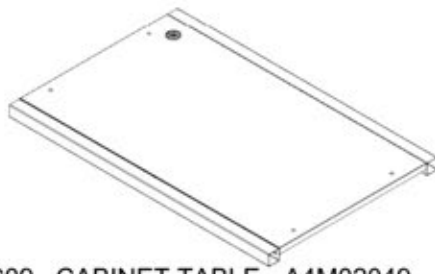
C09 CABINET TABLE - A4M02049 (x1) 2 3/8"x25"x38 7/16" (60x635x977)
