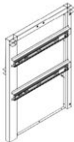
C08 CABINET PANEL - A4M02048 (x1) 4 1/8"x25"x35 7/16" (105x635x900)
