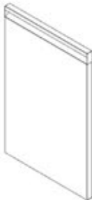
D03 DOOR PANEL - A4M02067 (x1) 7/8"x14 5/8"x22 7/16" (22x372x570)
