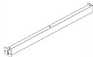
R01 RAFTER - A4M02020 (x4) 3 1/8"x3 15/16"x45 1/16" (80x100x1144)
