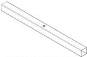
T02 UPRIGHT TUBE - A4M02104 (x1) 1 9/16"x1 9/16"x22 11/16" (40x40x576)
