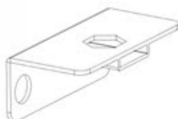
A05 HOSE CLAMP - A4M02258 (x1) 1 3/16"x1 9/16"x 3 1/8" (30x40x80)
