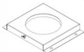
A12 PROPANE TANK HOLDER - A4M02028 (x1) 1 5/8"x11 13/16"x14 9/16" (41x300x370)
