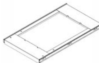
A04 7 GALLON TRASH CAN HOLDER - A4M02074 (x1) 1 1/4"x12 9/16"x21 5/8" (32x319.5x550)
