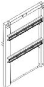
C08 CABINET PANEL - A4M02048 (x1) 4 1/8"x25"x35 7/16" (105x635x900)
