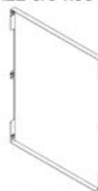
BP04 BACK PANEL - A4M02054 (x1) 1 3/16"x25 13/16"x33 7/8" (30x656x860)
