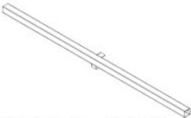
F13 TABLE RAIL - A4M02274 (x1) 2 3/8"x2 3/4"x53 5/16" (60x70x1354)
