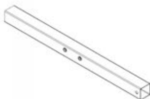
F06 TABLE TUBE SUPPORT - A4M02205 (x1) 1 9/16"x1 9/16"x21 7/8" (40x40x555)
