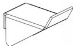
A06 ADJUSTABLE SHELF TAB - A4M02077 (x8) 11/16"x7/8"x1 3/16" (17x22x31)
