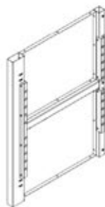
C05 CABINET PANEL - A4M02045 (x1) 2 3/16"x25"x33 7/8" (56x635x860)
