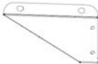
B09 CORBEL - A4M02042 (x1) 1 7/16"x6 11/16"x11 1/8" (36x170x282)
