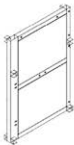
C02 CABINET PANEL - A4M02017 (x1) 3 15/16"x25"x37" (100x635x940)
