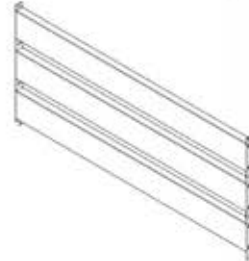
B10 BACK PANEL - A4M02043 (x2) 1 7/16"x22 11/16"x49 5/8" (36x576.5x1261)
