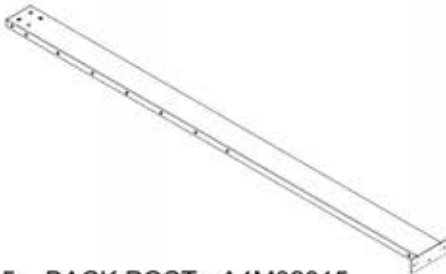
P05 BACK POST - A4M02015 (x1) 2 5/8"x7 7/8"x88 3/4" (66x200x2254)
