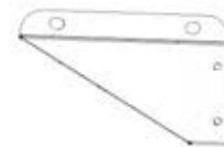
B09 CORBEL - A4M02042 (x1) 1 7/16"x6 11/16"x11 1/8" (36x170x282)
