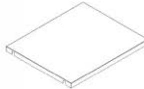
F10 FLOOR PANEL - A4M02208 (x1) 1 3/16"x18 3/8"x21 3/4" (30x467x553)
