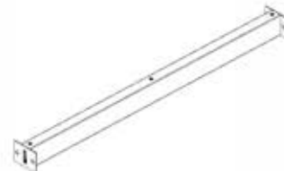
R01 RAFTER - A4M02020 (x4) 3 1/8"x3 15/16"x45 1/16" (80x100x1144)
