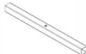
T02 UPRIGHT TUBE - A4M02104 (x1) 1 9/16"x1 9/16"x22 11/16" (40x40x576)
