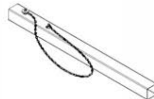
T03 UPRIGHT TUBE WITH MATCH HOLDER - A4M02404 (x1) 1 9/16"x1 9/16"x22 11/16" (40x40x576)
