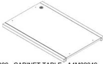
C09 CABINET TABLE - A4M02049 (x1) 2 3/8"x25"x38 7/16" (60x635x977)
