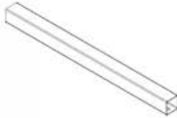
F04 FLOOR TUBE - A4M02203 (x2) 1 9/16"x1 9/16"x21 7/8" (40x40x555)
