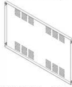
BP02 BACK PANEL - A4M02052 (x1) 1 3/16"x22 5/8"x38 7/16" (30x575x976)
