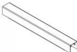
T01 TUBE - A4M02050 (x2) 1 9/16"x1 9/16"x14 7/8" (40x40x378)
