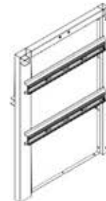
C08 CABINET PANEL - A4M02048 (x1) 4 1/8"x25"x35 7/16" (105x635x900)
