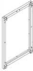
C01 CABINET PANEL - A4M02016 (x1) 2 3/4"x25"x38" (70x635x965)
