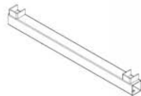
F09 BOTTOM FLOOR TUBE - A4M02210 (x1) 1 9/16"x2 3/8"x21 7/8" (40x60x555)
