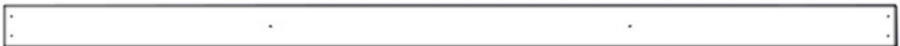
H03 LATTE AVANT - W4L18013 (x5) 15/16 po x 3 3/8 po x 70 11/16 po (24 x 86 x 1796)
