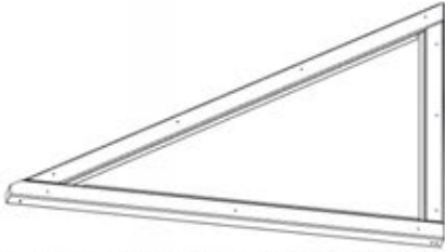
WP02 WINDOW PANEL ASSEMBLY - W2A03906 (x1) 1 7/16"x19 11/16"x32 11/16" (36x501x736)
