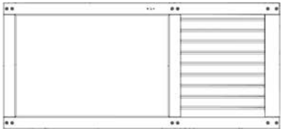
DA01 DOOR ASSEMBLY - W2A04009 (x1) 1 7/8"x36 9/16"x80" (48x928x2032)
