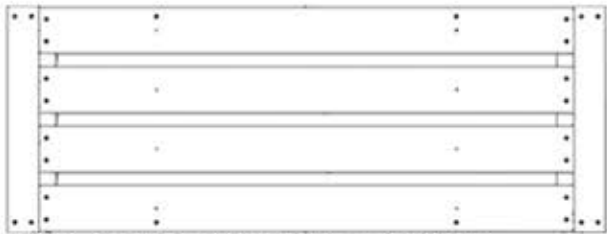
TB02 TABLE ASSEMBLY - W2A04152 (x1) 2 1/16"x16 1/16"x42 11/16" (52x408x1084)
