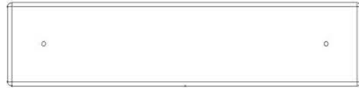
BH1-BOTTLE HOLD BOARD - W4L21182 (x2) 5/8"x2 3/8"x9 15/16" (16x60x250)
