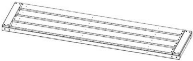
TP02 MID LONG TABLE ASSEMBLY - W2A03994 (x1) 2 1/16"x16"x60 1/16" (52x407x1406)
